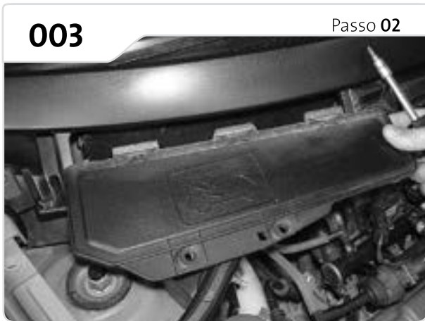
Remova a tampa puxando suavemente as travas.
